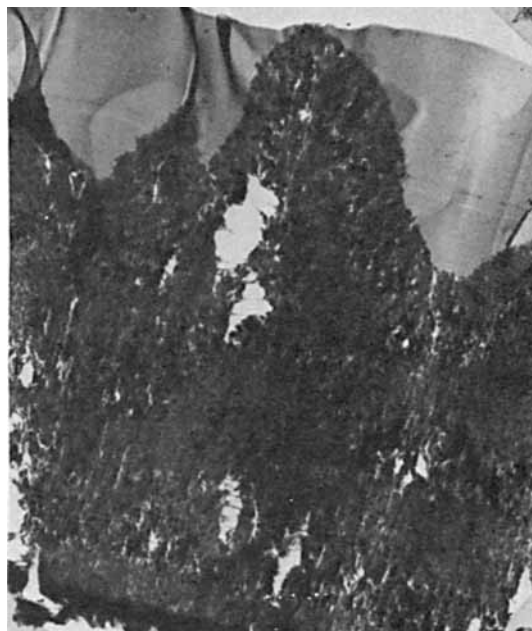
Fig. 11. Transmission electron micrograph of a cross section cut from a hazy deposit made at 190°C.
